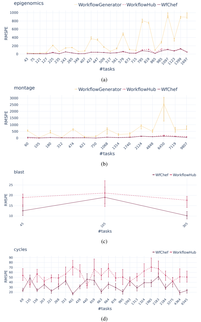
Figure 6: RMSPE of simulated task start dates for Epigenomics (a) and Montage (b), Blast (c) and Cycles (d) workflows instances. Points are average values. Error bars show the range between the third quartile (Q3) and the first quartile (Q1), and minimum and maximum values as black dots.
